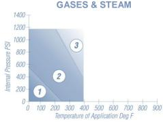
In area  $\Phi$ , the gasket material is suitable using common installation practices subject to chemical compatibility.
